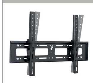
Flat Screen Wall Mount With Tilt For 32" up to 65" screens from VESA 200 x 100 up to 600 x 400
