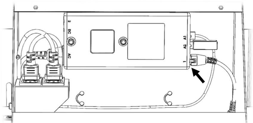
6. Plug the adapter into port 1 of the control box, then plug the motor lead into the adapter, next plug the 3.5mm jack from the anti-crush bumper into the adapter.
